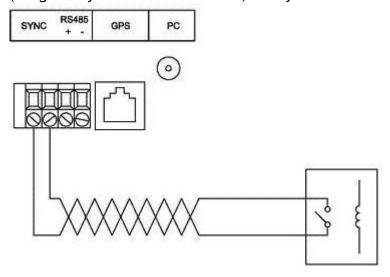
Verify Jumpers are "Closed" as shown for Sync Input. To access jumpers see page 3.
